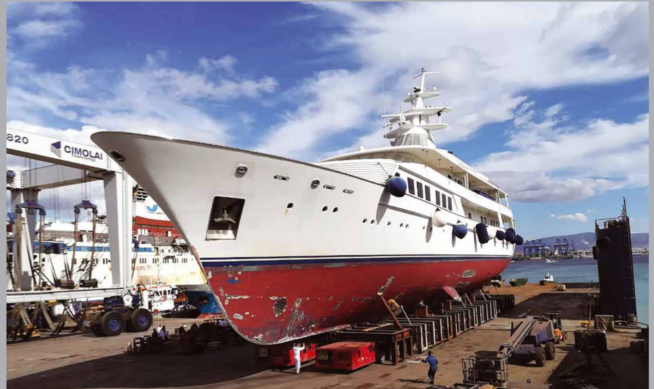
DRYDOCKING AND TRANSFER ASHORE OF A 65M YACHT BY BLOHM + VOSS
