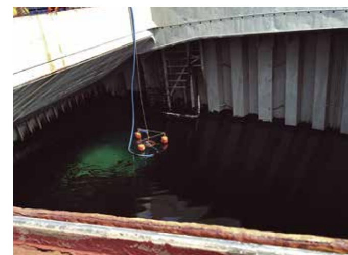
OIL RECOVERY DURING WRECK REFLOATING
